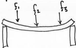
Hooke's law  $\rightsquigarrow$  the vertical displacements at those three points  $y_1, y_2, y_3$  are given by a linear transformation:
