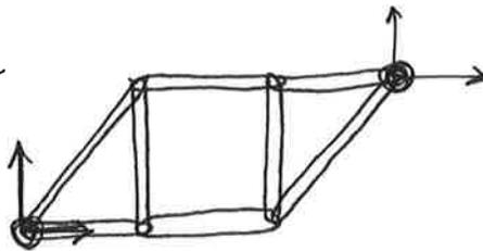
Find force at each joint given the forces at the two ends.
